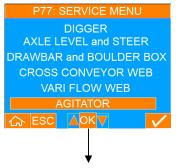
Select AGITATOR with up/down buttons and press OK.
