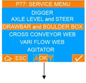
Select DRAWBAR and BOULDER BOX with up/down buttons and press OK.
