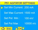
Select value you want to edit with up/down buttons and press OK. Change value with up/down buttons. Press OK to save.
