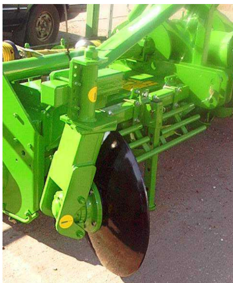
Fig 7:1a – 26" Diameter Heavy Duty Disc Openers
