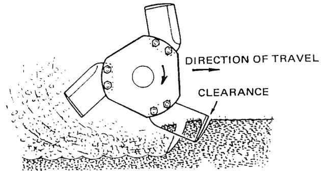
Correct blade setting showing clearance at back of blade.
