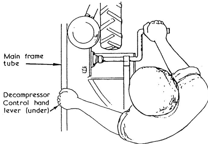
NOTE: In severe climatic conditions it may be necessary to oil prime the engine as described on page 24 of the engine manufacturer's handbook before repeating step 4.
