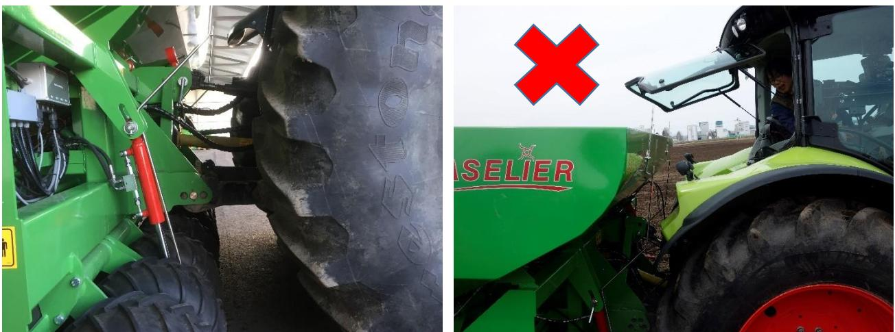
D. Adjust the lowering speed of the machine with the 3 point linkage to slow when the machine goes down.
